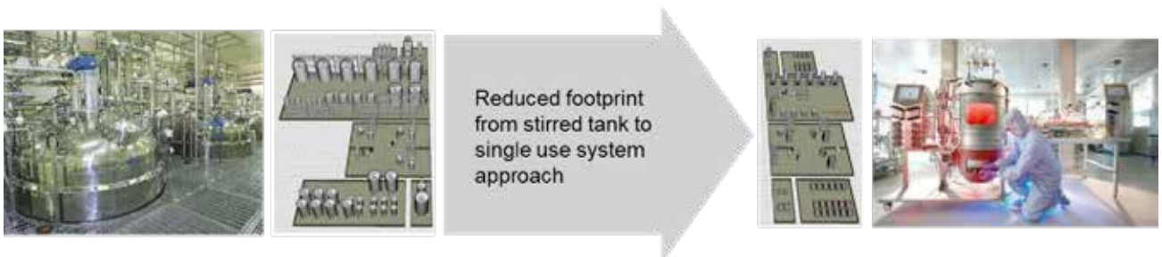
Figure 3: Reduced footprint: Stirred tank replaced by SUS. Reprinted from reference 3.
