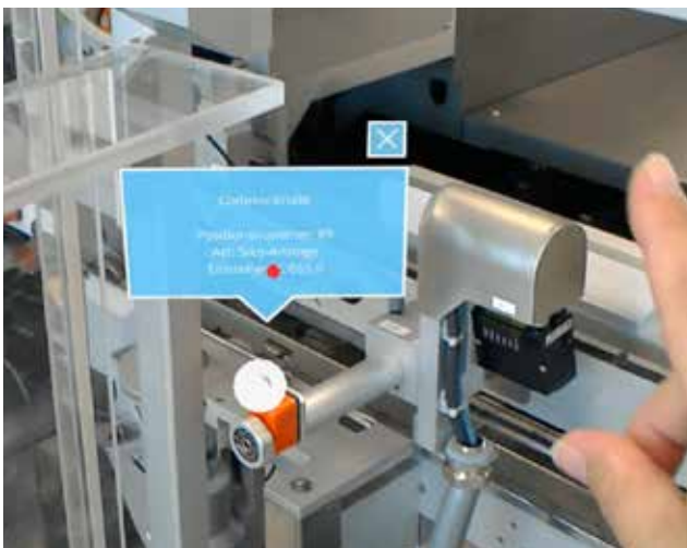
Figure 7: A worker at Merck Healthcare KGaA, in Mollet del Vallès, Spain, uses a mounted tablet with a heads-up display interface and touch control. Reprinted with permission from Merck.
